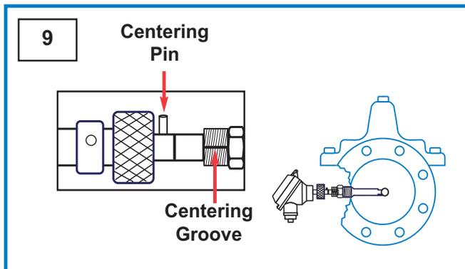
**Step 9:** Line-Up Centering Groove on straight threads with Centering Pin; push to seat o-ring
