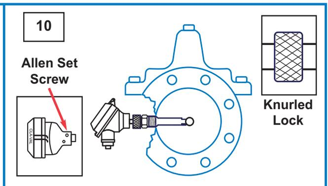
**Step 10:** **HAND TIGHTEN** Knurled Lock onto straight threads. Tighten Allen Set Screw with M3 Allen Wrench to lock Sensor Head Assembly.
