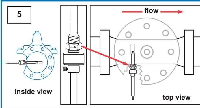
**Step 5:** Insert straightened Swivel Insert/Measurement Cylinder Assembly into valve, orient arrow on wrench flat to point downstream
