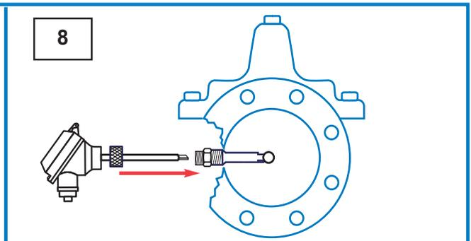
**Step 8:** Insert tip of e-FlowMeter Sensor/Head Assembly into Threaded Swivel Insert
