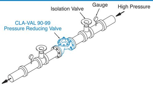
We recommend providing adequate space around valve for maintenance work
