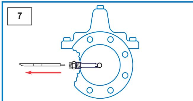
**Step 7:** Remove tool from Threaded Swivel Insert
