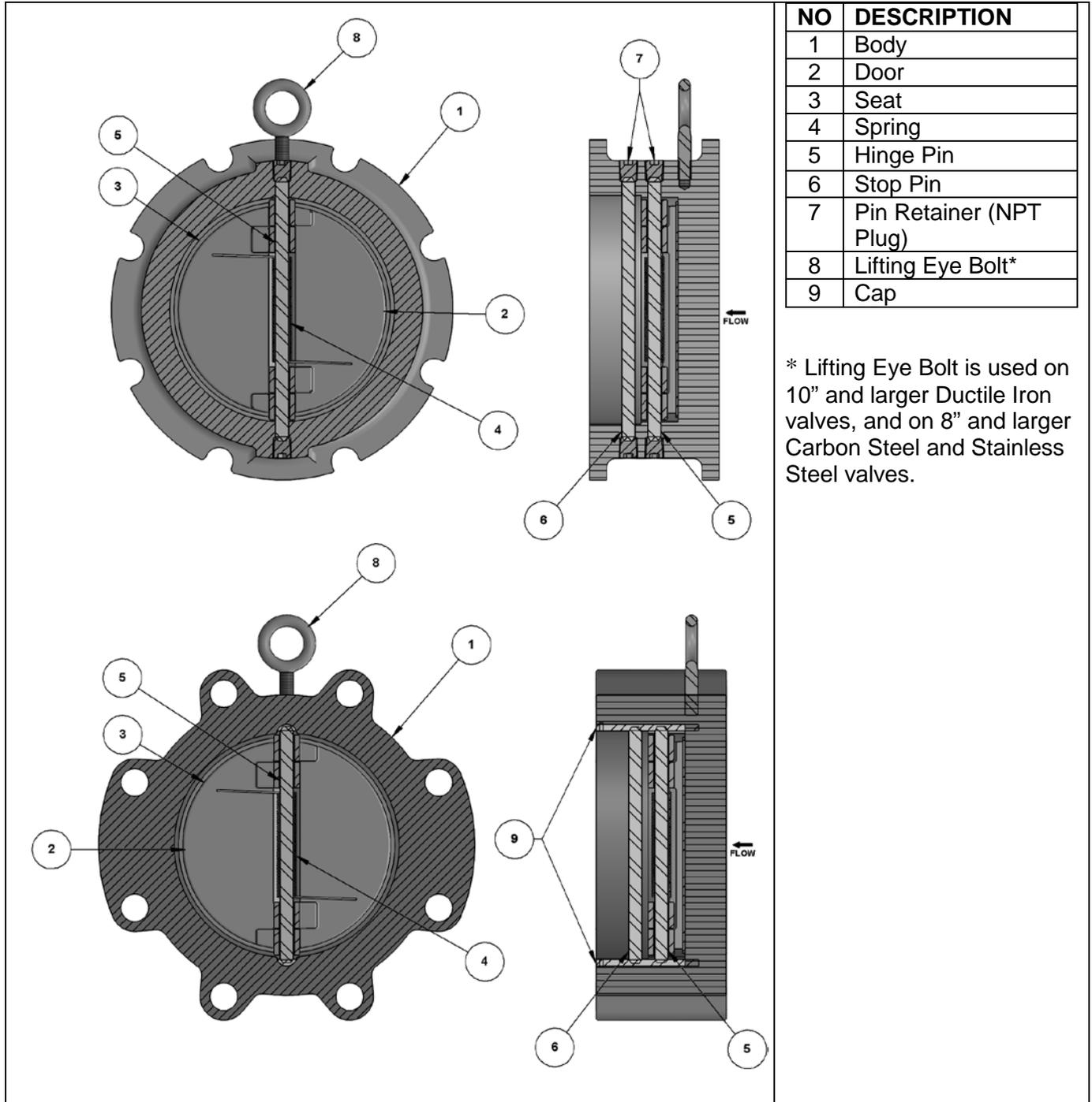
Figure 1 – 582 Series Two-Door Wafer Check Valve
