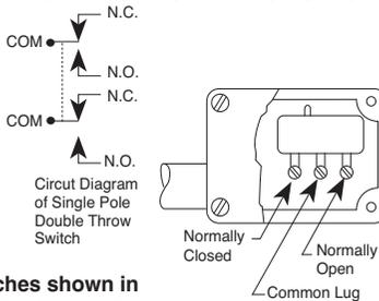
Switches shown in unactuated position.
