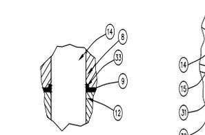
DIAPHRAGM WASHER SEAL DETAIL
