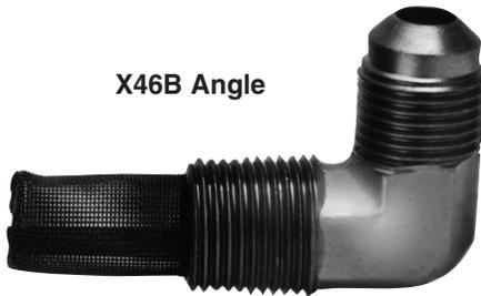
The X46 Flow Clean strainer operates on a velocity principle utilizing the circular "air foil" section to make it self cleaning. Impingement of particles is on the "leading edge" only. The low pressure area on the downstream side of the screen prevents foreign particles from clogging the screen. There is also a scouring action, due to eddy currents, which keeps most of the screen area clean.
