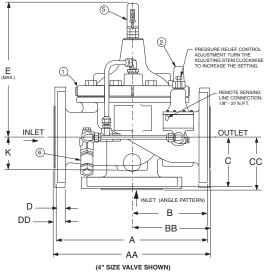
OPENING SPEED CONTROL ADJUSTMENT: TURN THE ADJUSTING SCREW CLOCKWISE TO MAKE THE MAIN VALVE OPEN SLOWER.
